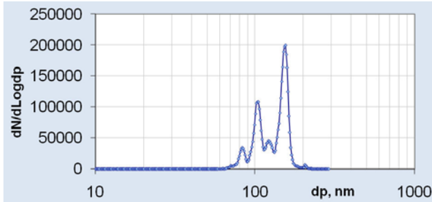
Figure 5. A typical PSD obtained with NaCl particles fractionated using the Naneum DMA model PMC500 configured for mobility equal to 150 nm for a singly-charged particle. The sample aerosol was charged with a K_r source and recorded with the NPS500 Nanoparticle Spectrometer neutralizer.
